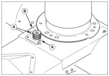
Figure 12. Discharge Chute Motor Adjustment A. Adjustment Screws B. Plastic Cover
